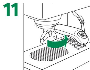
11 Insert filter basket into porta-filter and insert into group head, reattach cup-holder grid
